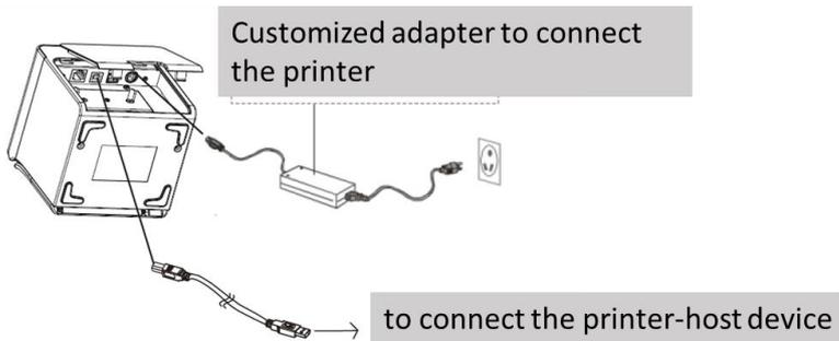
Please use the customized power adapter provided together with the printer. Connection as shown in above figure.
